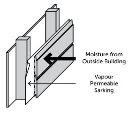
Figure 5 Vapour Permeable Layer
