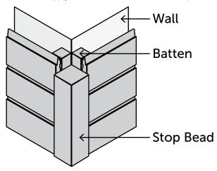
Figure 8 Cladding Corner Detail
