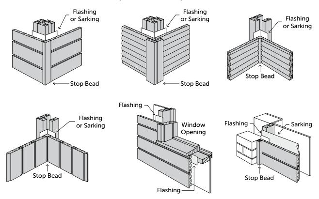
Figure 4 Typical Installation Details
