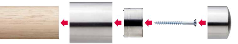
Use Porta Round 43mm dowel handrail Insert Porta Alignment Jig over the dowel, ensuring it is fully inserted against the end of the dowel. Take care not to mark the handrail Insert the connector (supplied with the fitting), pushing firmly, to engage the teeth. Pre-drill 3.0mm. Use a 10G x 50mm screw and fix firmly into place. Using Loctite® 680™ or equivalent high strength retaining compound, lightly coat the connector & inside fitting, and press into place until cured.
