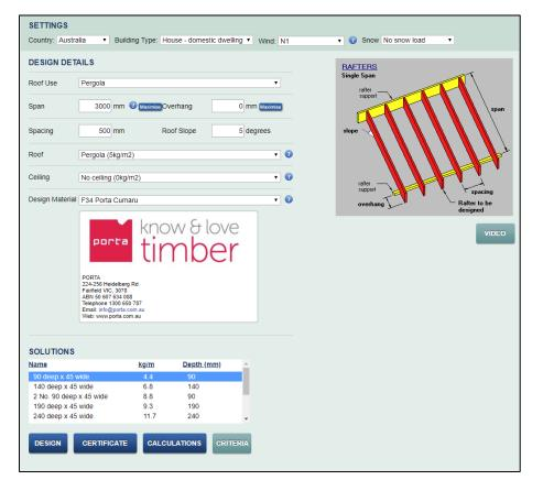
Click **CERIFICATE**. This will download the **SPANMAN DESIGN CERTIFICATE** for the section, providing all the necessary design information (for a building certificate) including deflections.
