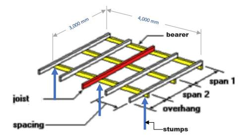
Distance between stumps: 2,000mm (span 1 & 2 for bearer beam). Overhang: 0mm Span across deck: 1,500mm (shown as span 1 & span 2 above)
