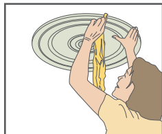
4. Fill any gaps with sealant & then wipe away excess.
