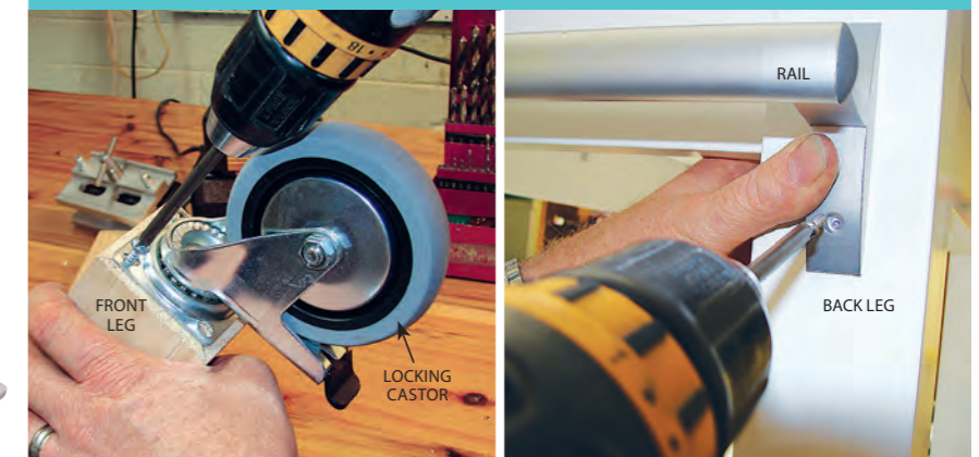
FOR CASTORS make 2mm diameter pilot holes in the front legs then attach 100mm locking castors, about $43 each, using the supplied screws.
